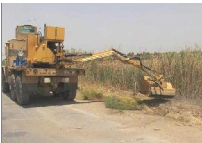
Figure 4. Flail mower mounted on an armored truck.
